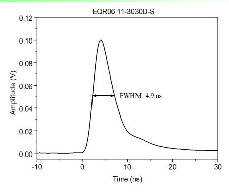
The single photoelectron pulse (amplified by a 60dB fast amplifier).
