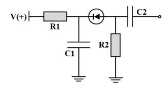
$R1 = 10 \text{ k}\Omega$   $R2 = 1 \text{ k}\Omega$  C1 = 100 nF C2 = 10 nF
