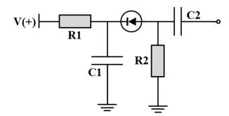
$R1 = 10 \text{ k}\Omega$   $R2 = 1 \text{ k}\Omega$  C1 = 100 nF C2 = 10 nF
