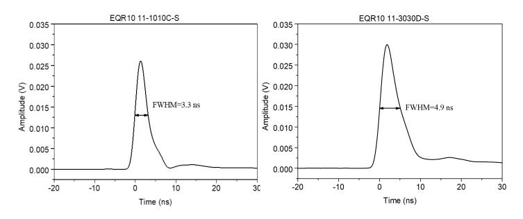
The single photoelectron pulse (amplified by a 40dB fast amplifier ).
