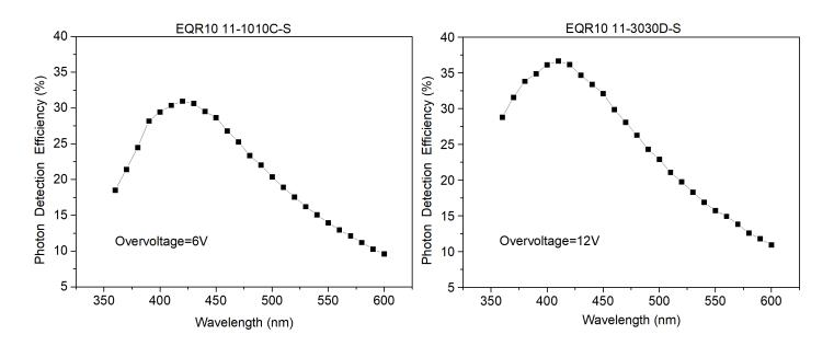
The PDE versus overvoltage and wavelength, deducted crosstalk and afterpulse and measured at 20  $^{\circ}\mathrm{C}$  .
